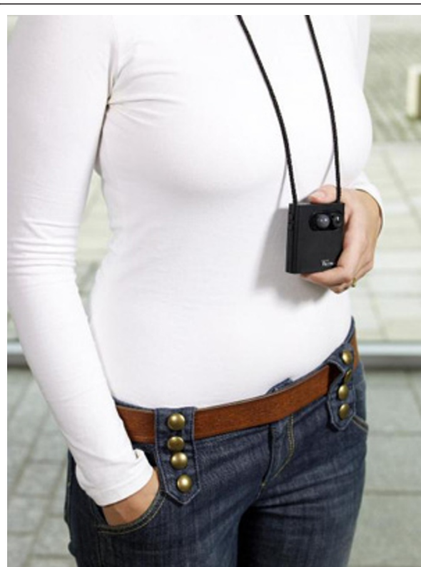
Figure 1 The Microsoft SenseCam digital camera. This wearable device weighs 175 g and passively captures approximately 3,600 first-person point-of-view digital images per typical day.
