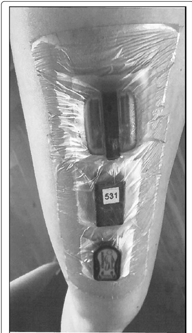
**Fig. 1** Illustration of accelerometer placement (top to bottom: Actigraph GT3X+, Axivity AX3, ActivPAL Micro) in a vertical line on the mid-section of the thigh. Accelerometers were placed approximately 2 cm apart and were attached directly to the skin using double sided tape. The order of the accelerometer placement was followed a randomized partial counterbalance design
